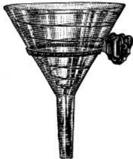
In filtering a liquid which contains a precipitate (unless the precipitate is designed to clear the liquid, as magnesia or pumice-stone are used) the liquid should be poured carefully off and filtered first, the precipitated portion being added after most of the liquid has passed through the filter; this makes the process more rapid.
