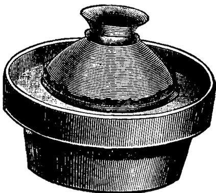
In pharmacy, dialysis is employed to separate what are known as *colloid* (glue-like) substances, from their combination in solution with crystallizable substances. This is accomplished by means of an apparatus called a Dialyzer, a simple form of which is here illustrated.
